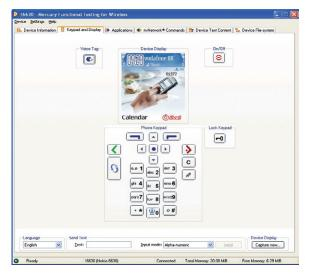
Mercury Functional Testing for Wireless enables testers to connect, control, and display the software from a Symbian OS phone and perform multitudes of functional tests.
